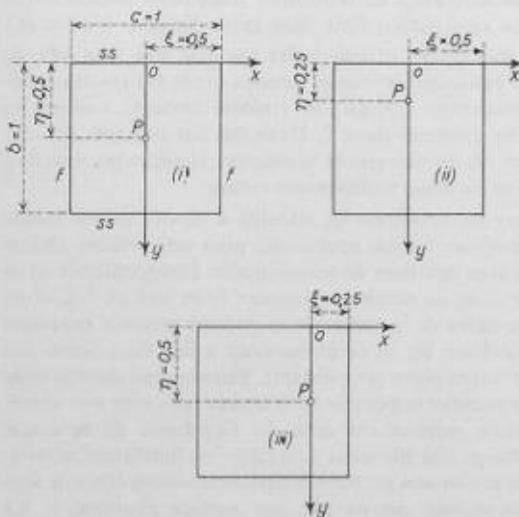
Fig. 5. Position of load and orthotropic plate dimension for numerical examples when two opposite edges are simply supported and remaining edges are free.
