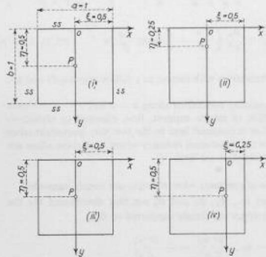
Fig. 3. Position of load and orthotropic plate dimensions for numerical examples where all edges are simply supported. Note:  $D_x = 2D$ ,  $D_y = D$  in cases (iii) and (iv). ss — simply supported
