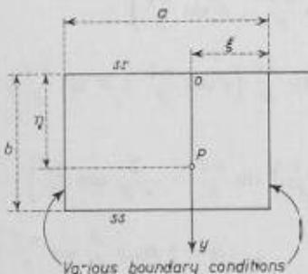
Fig. 2. Rectangular plate under concentrated load.
