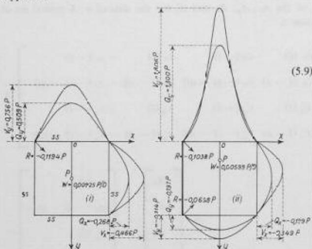
Fig. 4. Numerical values for examples where all edges are simply supported. The corner reactions  $R$  are given by  $\pm 2 M_{xy}$ .  $R$  positive indicates opposite sense to  $P$ .  $a = b = 1$ ,  $D_x = D$ ,  $D_y = 2D$ ,  $D_1 = 0.15 D$ ,  $D_{xy} = 0.425 D$
