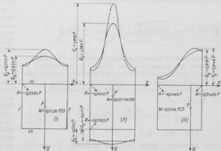
Fig. 6. Numerical values for examples when two opposite edges are simply supported and remaining edges are free. The corner reactions  $R$  are given by  $\pm 2M_{xy}/P$ .  $R$  positive indicates opposite sense to  $P$ .  $a = b = 1$ ,  $D_x = D$ ,  $D_y = 2D$ ,  $D_1 = 0,15 D$ ,  $D_{xy} = 0,425 D$ .
