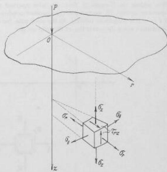
Fig. 5. The stress components in Boussinesq's solution for the semi-infinite elastic solid
