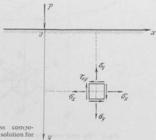
Fig. 1. The stress components in Flamant's solution for the elastic half-plane
