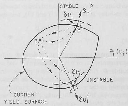
Fig. 3. Overall stability and instability of an elastic-plastic continuum or structure
