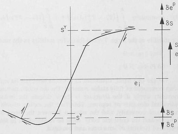
Fig. 2. One-dimensional example of normality and convexity (stable in tension, unstable in compression). Note that  $S^Y$  in tension and  $S^Y$  in compression are independent points on different yield surfaces
