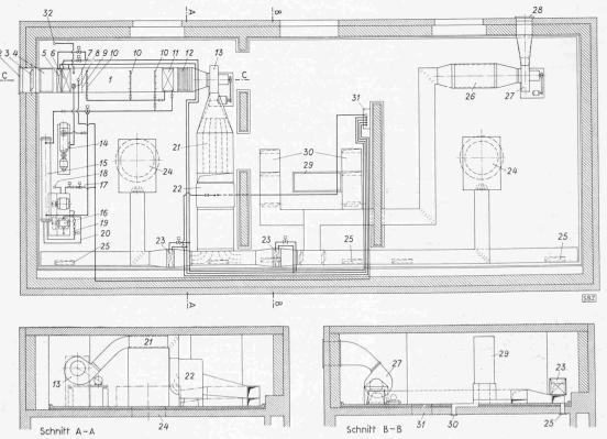
${\bf Bild}\ 2.\ {\bf Ventilations-und}\ {\bf klimatische}\ {\bf Einrichtungen}\ {\bf im}\ {\bf Spital}\ {\bf Grenchen},\ {\bf Masstab}\ 1:100.$
