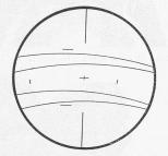
${\tt Horizontal distanz} = 100 \times 22.7 = 22.7 \; {\tt m}$ Höhendifferenz  $= 20 \times 16.5 = 3.30 \text{ m}$
