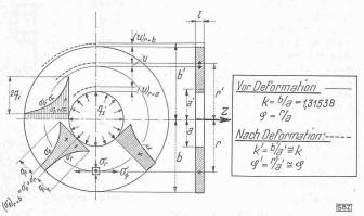
Abb. 5. Abmessungen des Eichrings in mm: b = 85.5; a = 65.0; l = 6.72
