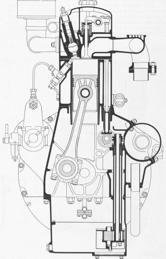
Abb. 1. F. B. W.-Dieselmotor,  $n=1800~\mathrm{U/min},~N_e=15~\mathrm{PS/Zyl.}-1:7$
