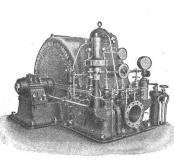
Patent - Freistrahl - Turbine. 2500 HP, 300 Meter.
