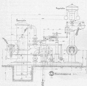
Fig. 10. Regulator Servomotor Ganz 1:40.
