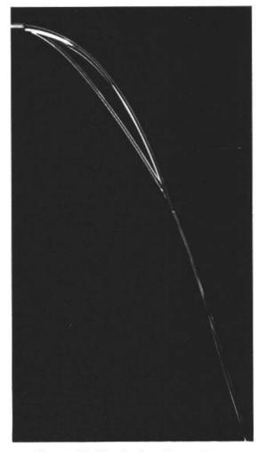
Fig. 4. Jet laminaire, Re = 260.
