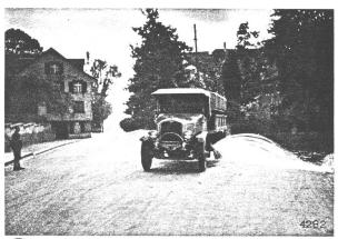
APROSEUSE SANS POMPE. SPRENGWAGEN JHNE PUMPE. WATERING WAGON WITHOUT PUMP.
