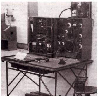
Figure 29: Station de radio lourde portable TS 18/25 (1927-1956).
