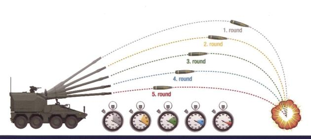
IMPACT TIME WITHIN 2 SECONDS / E.G. FIRING DISTANCE 12,000 m
