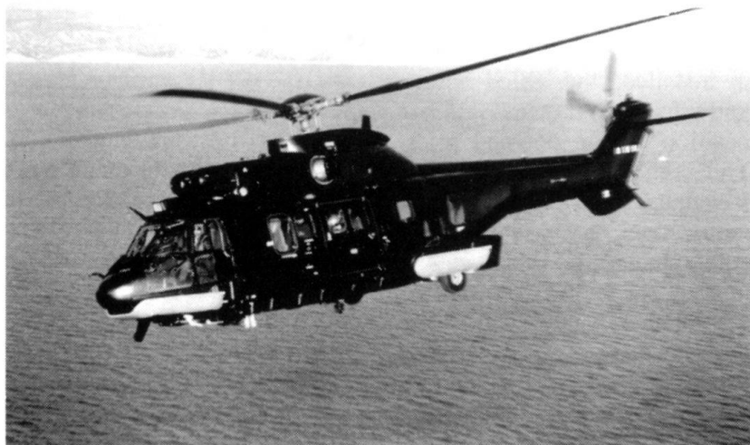
Versatile par excellence, the AS 532 U2 offers a large cabine. Its extended range and its integrated navigation systems make it a SAR and combat/SAR helicopter perfectly suited for today's requirements (day/night missions).
