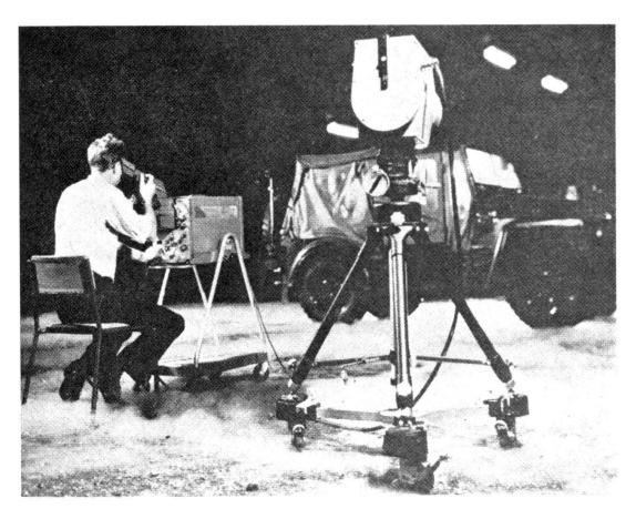
Figure 2. — Appareil AGA Thermovision.
