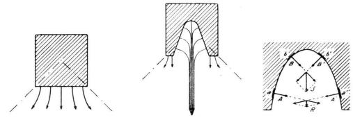
Fig. 1a. — Charge normale. Fig. 1b. — Charge creuse.
