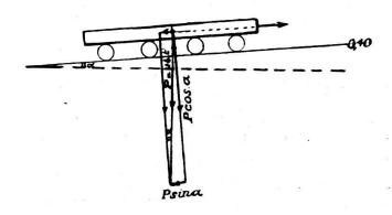
Fig. 2 Résistance due aux rampes
