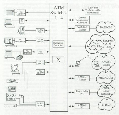
The environment of Exploit - an ATM Testbed
