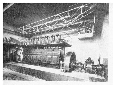
MOTEUR DIESEL 4 TEMPS 8 CYL. 2.500 CV.
