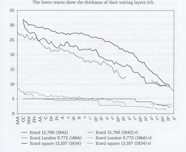
and then a steeper one to  $g^4$  (8.9 mm). The voicing layer is at 5 mm from CC to  $c^3$ , 4 mm to  $a^3$ , then (hand?) tapers to 2 mm at  $g^4$ .
