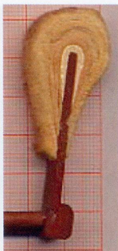
Illustration 4. Hammer from grand piano no. 1,232 by Pleyel et Cie., Paris April 1829 (RC M. Lambert) (private collection, France)
