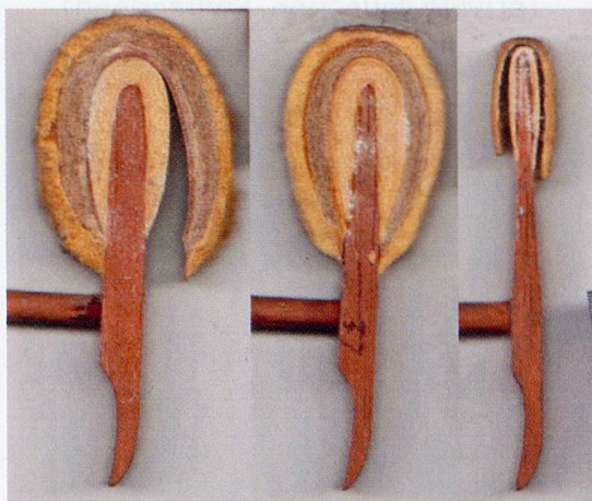
Illustration 23. Hammers for CC#, c 1 , g 4 , grand piano no. 11,126 by Pleyel et Cie, Paris October 1844 (RC Mr. Magnier, Moulins) (private collection, France)
