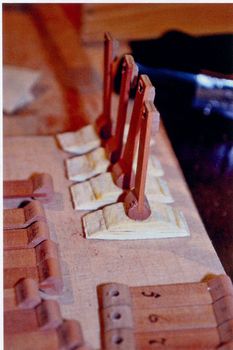
Illustration 29. Method for covering under-layers in leather (author's fac-simile, Erard 1802)
