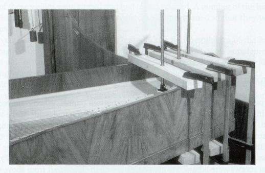
Figure 7: Clamping system devised by author to reglue bass bridge. As pressure is exerted on the bridge from above, the soundboard is supported from below by Jorgensen veneer press screws.
