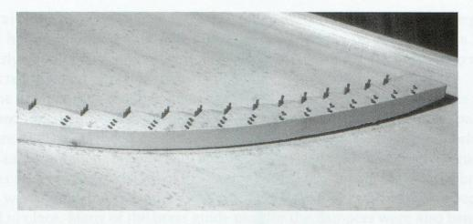
Figure 6: Detail of unglued section of bass bridge.
