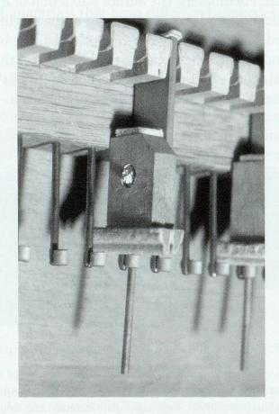
Figure 4: Detail of corroded lead weights in bass dampers.
