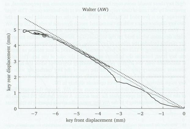
toward the front of the DS key. Measuring at rear, balance, and front positions these dimensions are: AW key -19, 18, 18 mm; DS key -16, 16, 11 mm. The stiffness of a beam in bending is related to the cube of its thickness, so the effect of tapering on key deformation during strong playing can be quite significant.
