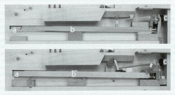
Figure 3: Bichord string model shown with DS (top) and AW (bottom) action model in correct configuration for observing experimental key strikes:
