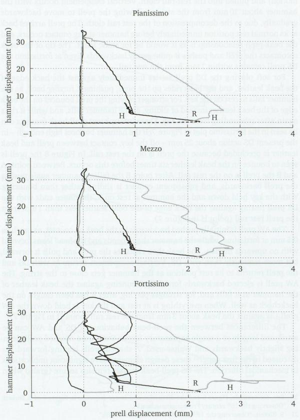
Figure 8: Horizontal displacement history of prell (black) for DS and AW with fortissimo dynamic level. Vertical displacement of hammer (grey) also shown (note cm used for visual clarity). Between points labelled A and B the high hammer and at-rest prell preclude beak-prell contact. Axes scales are the same for each subplot. Time zero is maximum string excursion.
