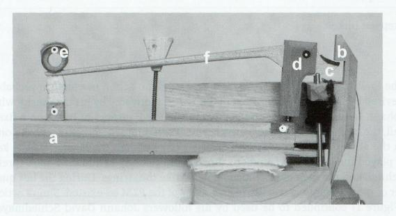
Figure 1: Stein-type PZM action model used for experimental observation, based on a 1794 JD Schiedmayer piano: a) key; b) prell; c) hammer beak; d) kapsel; e) hammer; f) hammer shank. The damper lifter is also seen behind.
