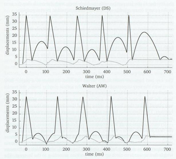
the hammer, cause drag on the key response while it is being depressed. The backcheck is therefore responsible for the irregularity of the note timing, and, in a less well-regulated action can also cause missed repeated notes. This does not happen in an action of the Stein type with no backcheck to interfere.
