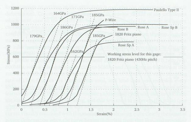
Figure 7. Stress-strain tensile curves from testing 0.68mm dia. wire samples. All elongations at breakage are approximately uniform except for the two samples indicated in bold, which broke in the gage length.
