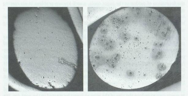
Figure 3. Optical microscope sectional views (x100): (L) historical iron wire sample (1820 Pape piano); (R) 0.1% P-wire sample. Note the historical sample is more free of inclusions.
