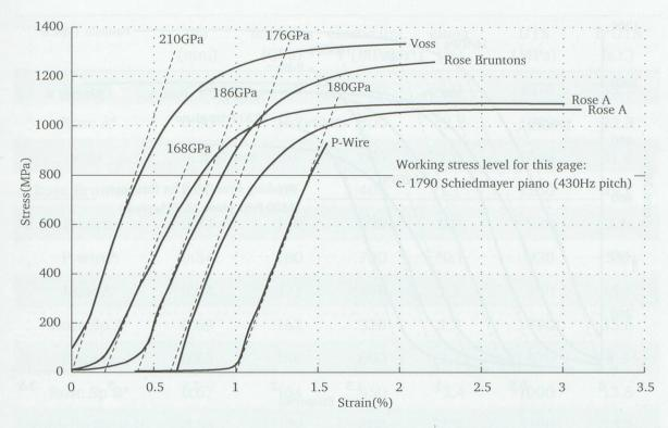
Figure 6. Stress-strain tensile curves from testing 0.34mm dia. wire samples. All elongations at breakage are approximately uniform except for the sample indicated in bold, which broke in the gage length (a test result is also shown from another sample of this material (0.49mm dia.) which did not break in the gage.)
