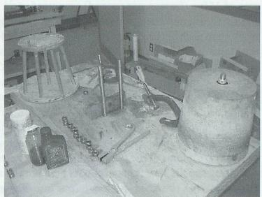
Figure 5. Powered ripping bench; hand-operated wire drawing bench (tungsten-carbide dies are seen in the foreground).
