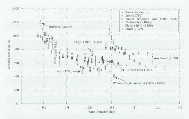
Figure 8. Working stress related to ferrous wire gage diameters on harpsichords and pianos.
