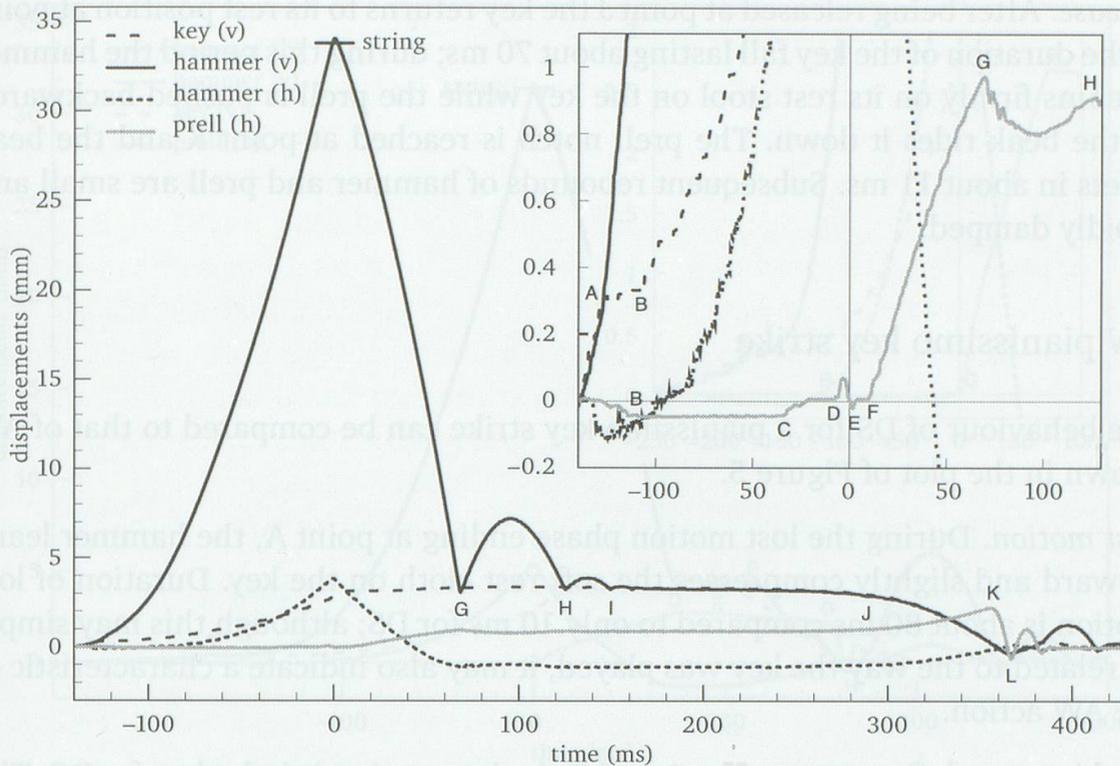
Figure 4: Vertical (v) and horizontal (h) displacements (mm) of hammer, key, and prell for DS pianissimo key strike. Time zero is maximum string deflection.
