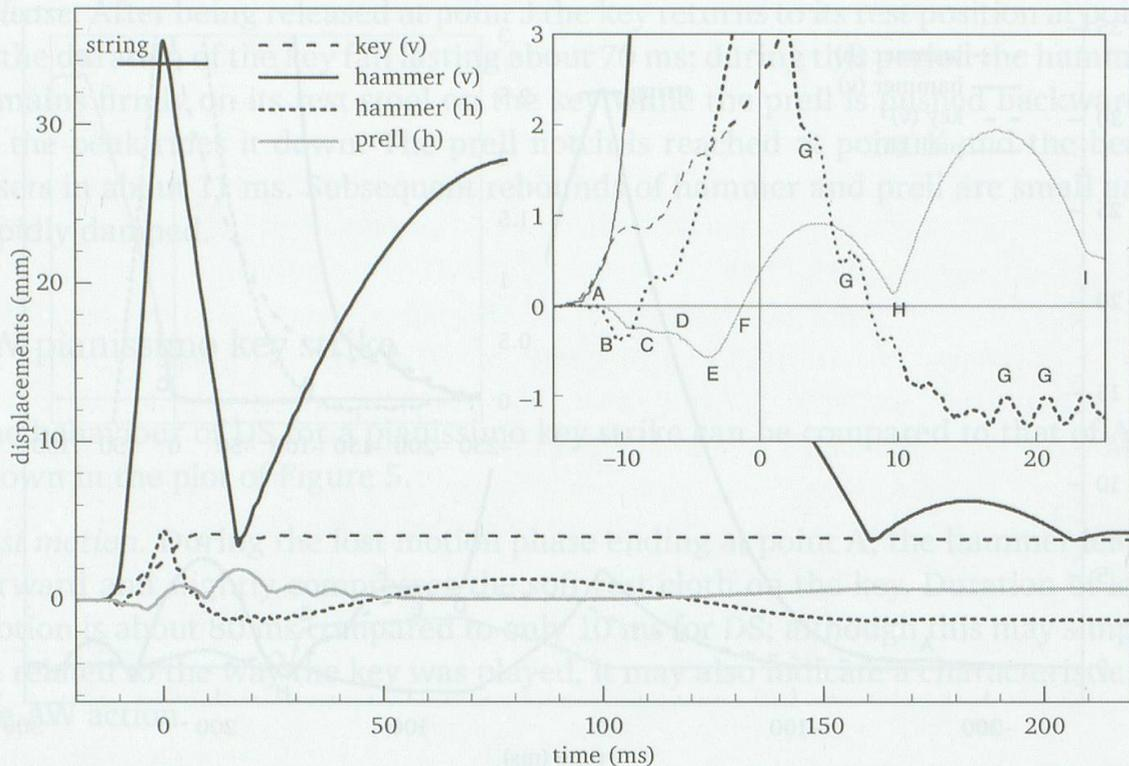
Figure 6: Vertical (v) and horizontal (h) displacements (mm) of hammer, key, and prell for DS forte key strike. Time zero is maximum string deflection. Rest position of string is marked.
