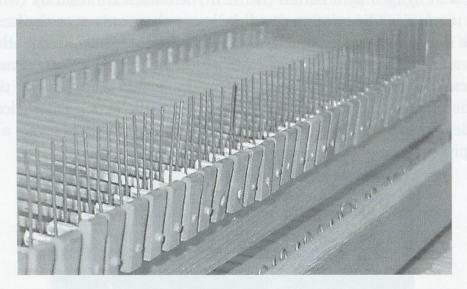
Illustration 11: The wooden hammers (with no covering of leather) in the 1777 *Vis-à-vis*. The vertical wires projecting out of the hammer rest rail act to guide the hammers as they rise. At the top and to the left the hammer rail is visible. At the bottom and to the right the pins (with a loop at the top) that secure the key levers where they are hinged at the rear (as on many organs) are just visible.
