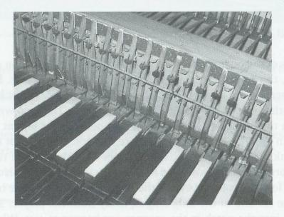
Illustration 9: The escapement hoppers in the action of the piano of the 1777 *Vis-à-vis*. Some of the hammer shanks with their hammers can also be seen beyond the pivot rail in the top right-hand corner of the photograph. Some of the beaks in their notches can be seen to the left. The felt bushings for the escapement hopper springs are not original. The springs would have fitted directly in the grooves in the hoppers. The little tongues between the hoppers hold the hammer pivot wire in place.
