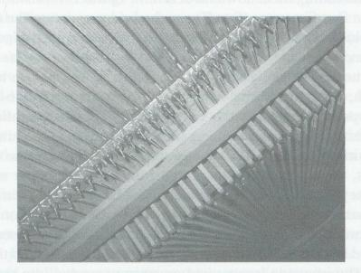
Illustration 13: Some of the squares at the harpsichord end of the 1777 *Vis-à-vis*. The undersides of the distal ends of the third keyboard are visible at the top left. The leather buttons on the rods screwed into them pull up the horizontal arms of the squares. The pivots of the squares are hidden behind the diagonal beam but the vertical arms and where they are attached to the trackers are visible below the beam. The converging trackers are also visible, disappearing into the gloom.
