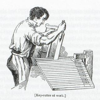
Figure 5: A key cutter at Broadwood's factory: illustration to George Dodd's article 'A Visit to a Piano-forte Factory', The Penny Magazine, April 1842.
