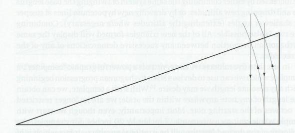
Figure 1b – Dividing the base line into proportional units.
