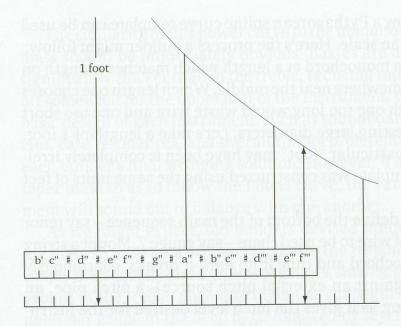
Figure 7 – Using the note ruler to find the length of  $f^{\prime\prime\prime}$  on the template.
