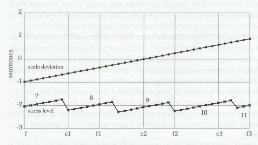
Chart 9 – Inequality of stress levels caused by using progressively smaller string diameters (gauge 7 to 11) in a non-Pythagorean Main Sequence (octave ratio 1:1.93).
