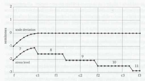
Chart 8 – Inequality of stress levels caused by using progressively smaller string diameters (gauge 7 to 11) in a Pythagorean Main Sequence.
