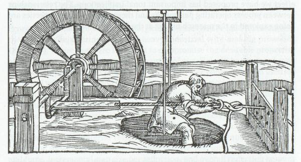
Figure 6. Ripping the iron rods to coarse wire using water power (from Biringuccio, 1540).
