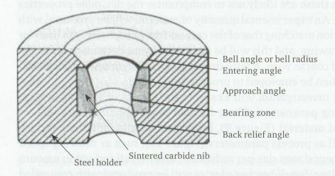
Figure 9. A modern wire-drawing die.
