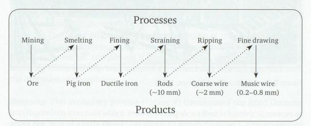
Figure 1. Historical industrial processes and intermediate products in iron wire manufacture.
