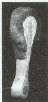
b) Felt-covered hammer by Pape, c. 1825. The outer layer is impregnated with a green solution against moth attack.
