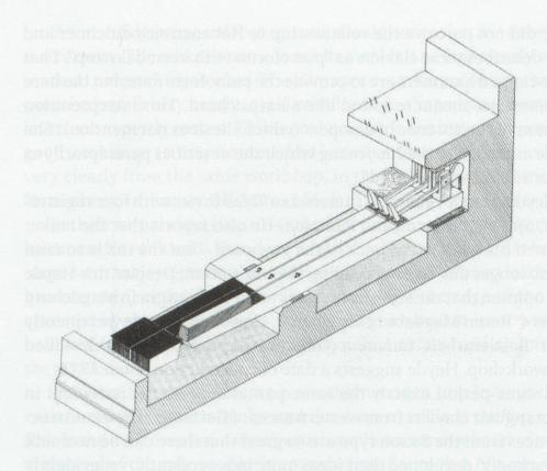
Figure 5. Flip Action (or retro *Prellmechanik*) with bare wooden hammers and without dampers.
