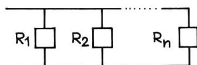
$$\frac{1}{R_{\text{tot}}} = \frac{1}{R_1} + \frac{1}{R_2} + \dots + \frac{1}{R_n}$$
