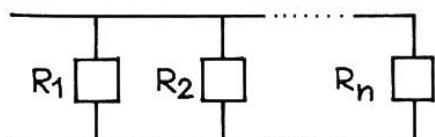
$$\frac{1}{R_{\text{tot}}} = \frac{1}{R_1} + \frac{1}{R_2} + \dots + \frac{1}{R_n}$$
