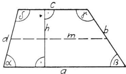
$$u = a + b + c + d \quad F = m \cdot h \quad \alpha + \beta + \gamma + \delta = 360^\circ$$
