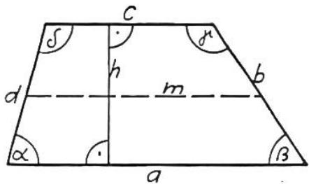
$$u = a + b + c + d \quad F = m \cdot h \quad \alpha + \beta + \gamma + \delta = 360^\circ$$
