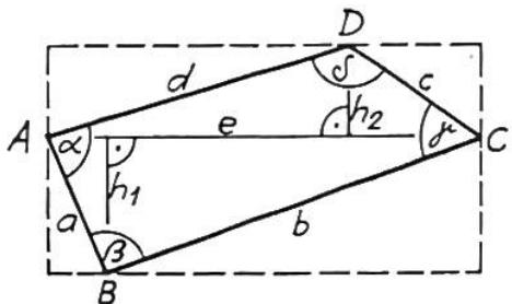
$$u = a + b + c + d \quad F = e \left( \frac{h_1 + h_2}{2} \right) \quad \alpha + \beta + \gamma + \delta = 360^\circ$$
