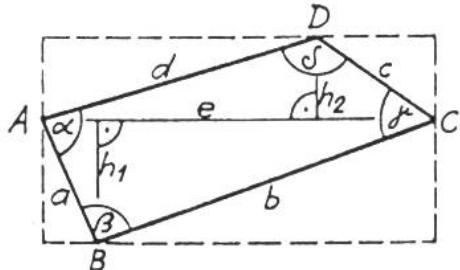
$$u = a + b + c + d \quad F = e \left( \frac{h_1 + h_2}{2} \right) \quad \alpha + \beta + \gamma + \delta = 360^\circ$$
