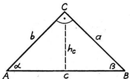
$$\alpha = \beta = 45^\circ \quad a = b = \frac{c}{\sqrt{2}} \quad c = a\sqrt{2} \quad h_c = \frac{c}{2}$$
