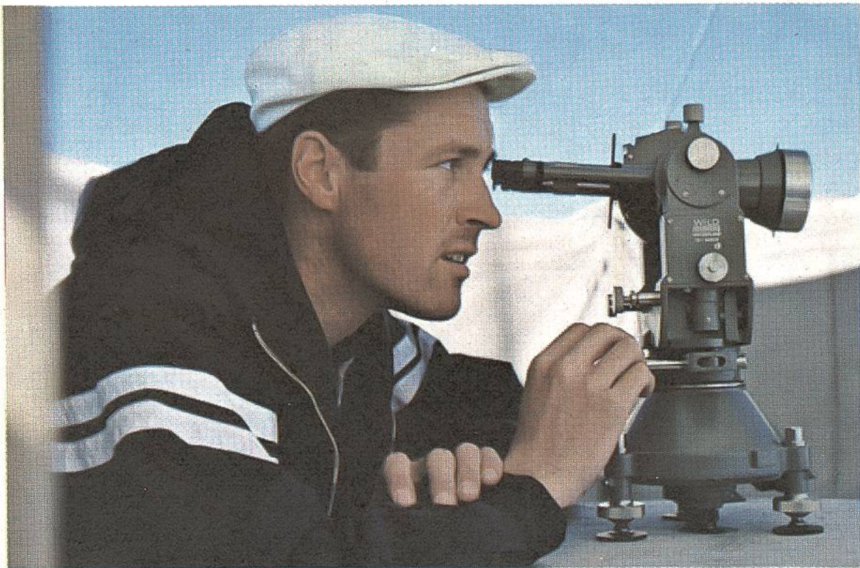
Winkelmessung am Theodolit.
