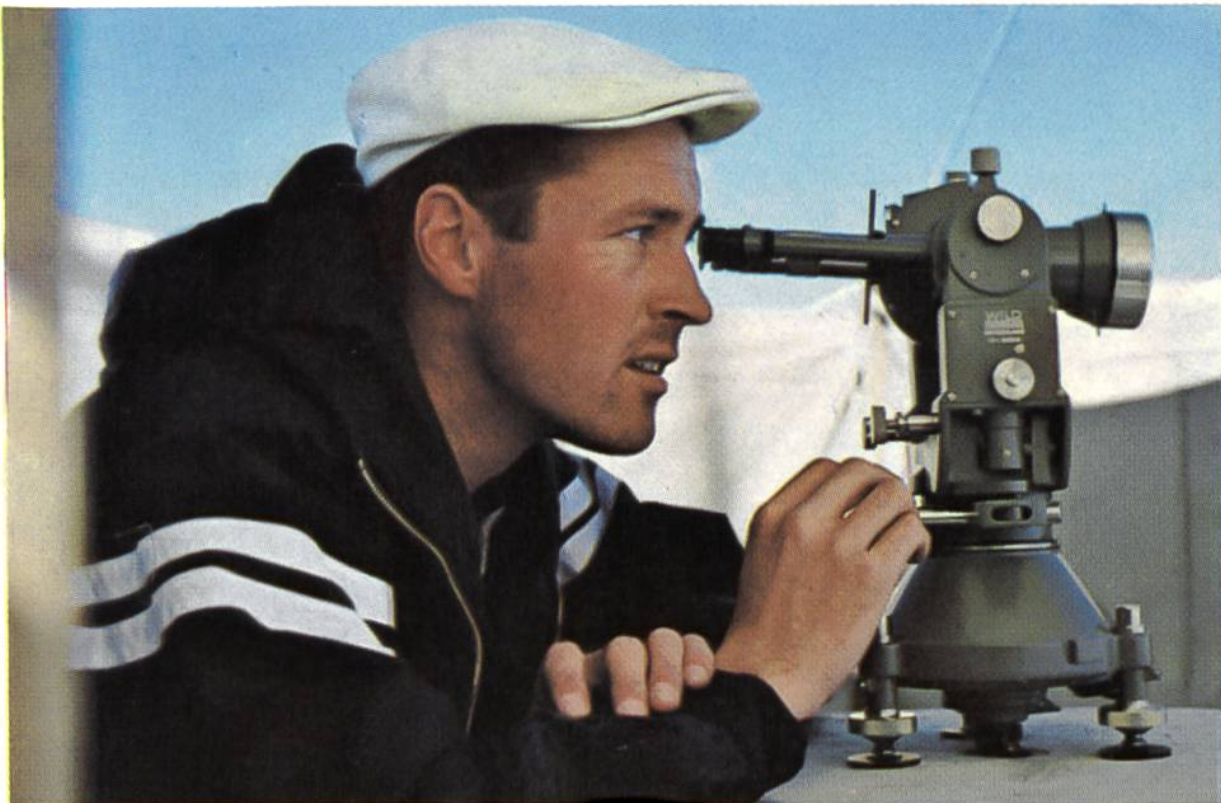
Winkelmessung am Theodolit.
