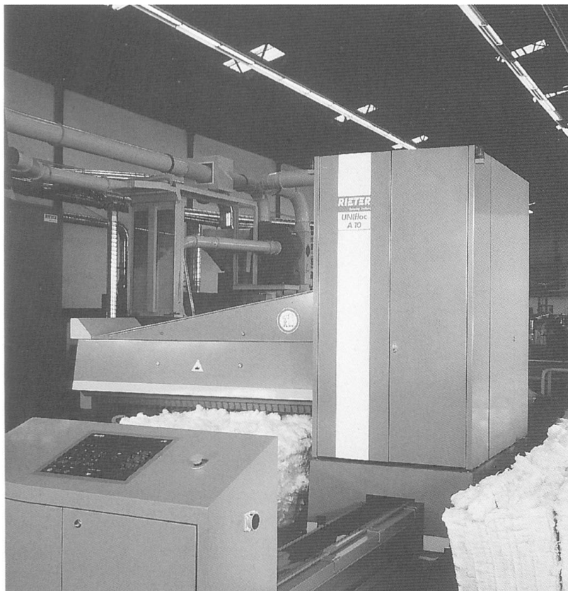
UNIfloc bale opening machines reduce the raw material into flocks of small size.
