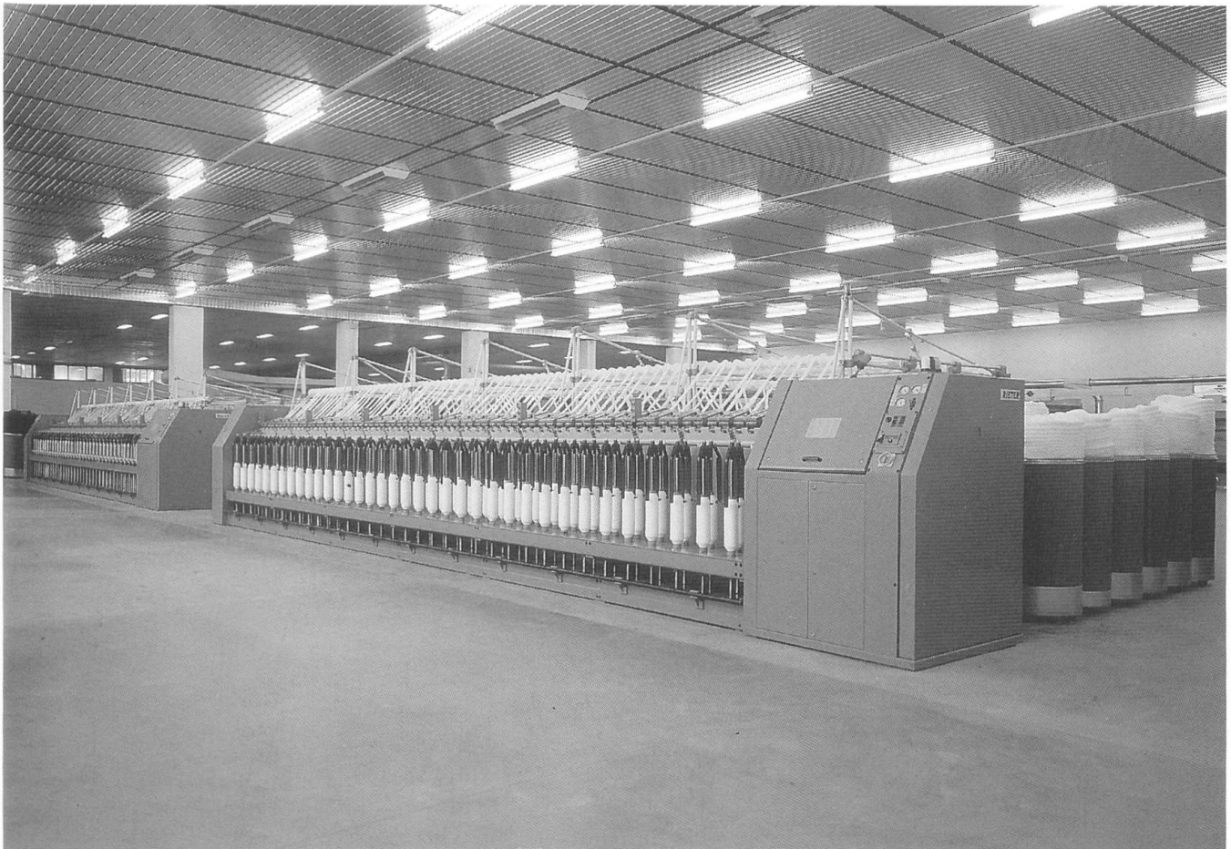
F1/1a speedframe with 355x178 mm (14 in. x 7 in.) packages and cast aluminium flyers ca. 1990
