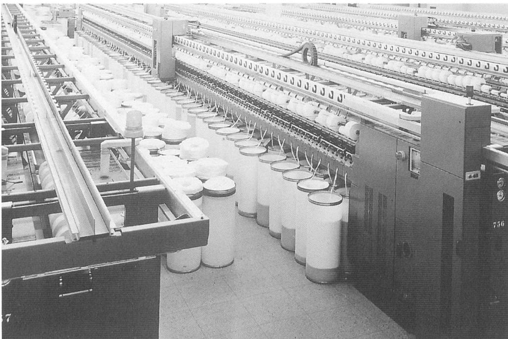
RU14-A achieved a maximum of 130 000 rpm with rotors only 30 mm in diameter and utilized the space under the machine especially efficiently with rectangular cans.
