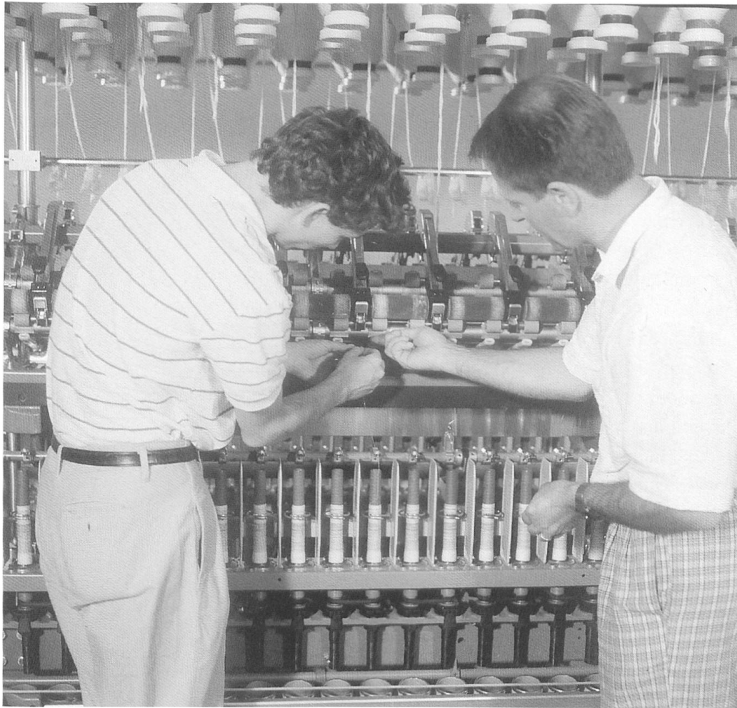
Training on the ring spinning drafting system
