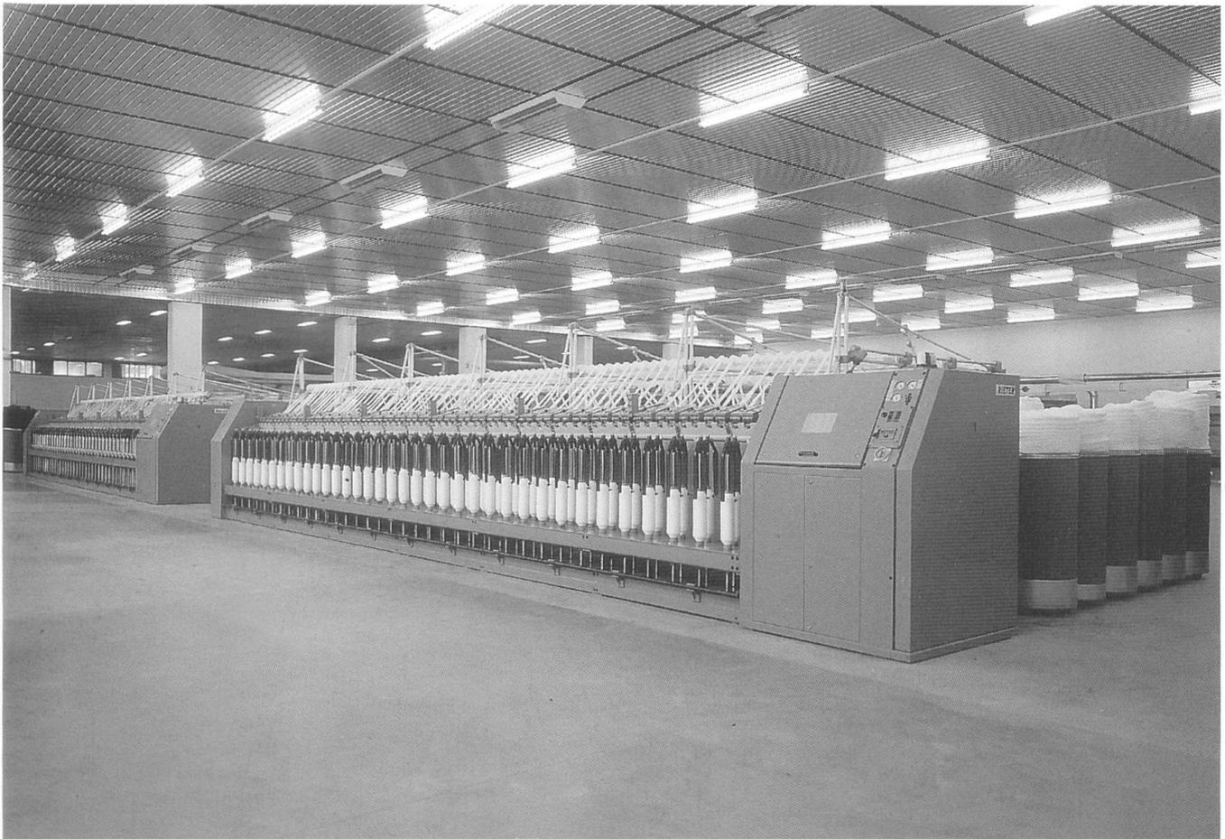
*F1/1a speedframe with 355x178 mm (14 in. x 7 in.) packages and cast aluminium flyers ca. 1990*
