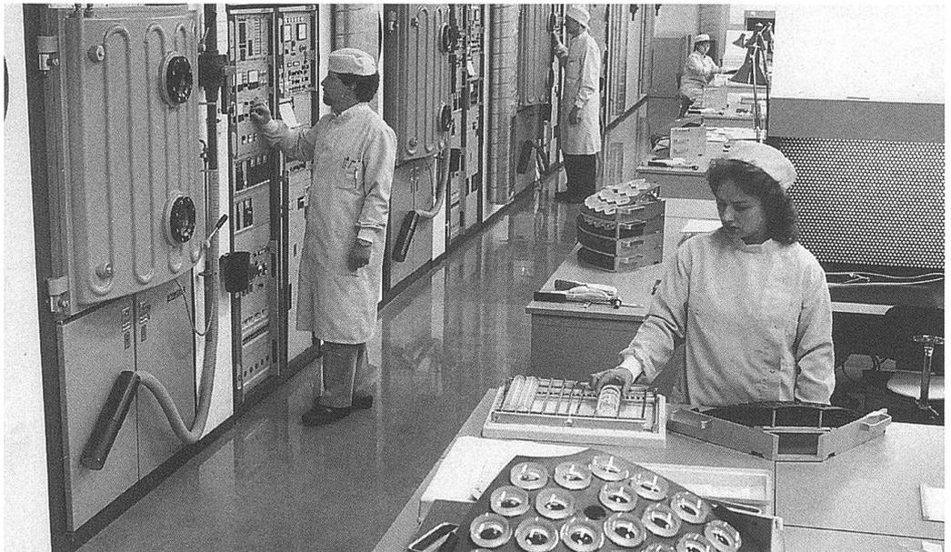
*Polishing of the lenses employed in the manufacture of optical equipment at Leica in Heerbrugg*
