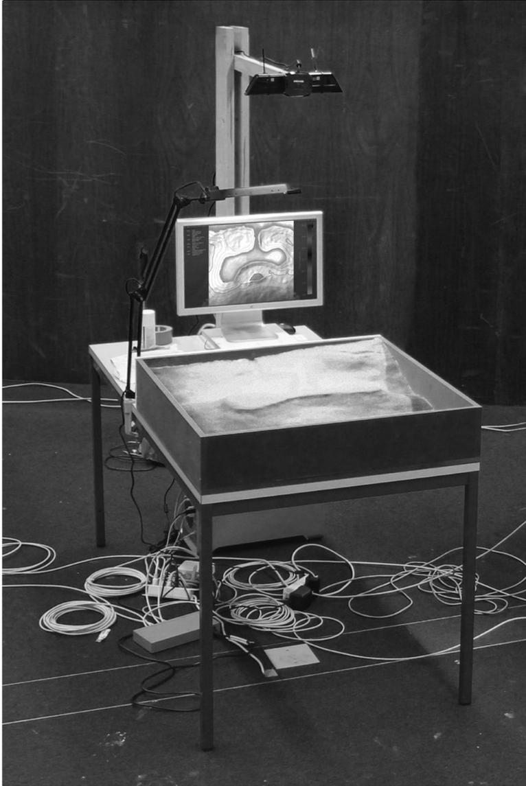
Table, sand box, 36 kg modeling sand, lamp, Microsoft Kinect 3D scanner, keyboard, HD monitor, Mac Pro. At the ETH Zurich, Switzerland, 2014.
