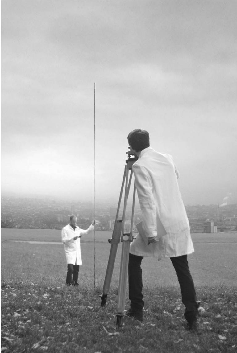
Automatic Leica Runner 24 optical level, wooden tripod, telescopic Grade Rod, Leica X310 laser distance meter, pencil, notebook. On the Käferberg in Zurich, Switzerland, 2015.
