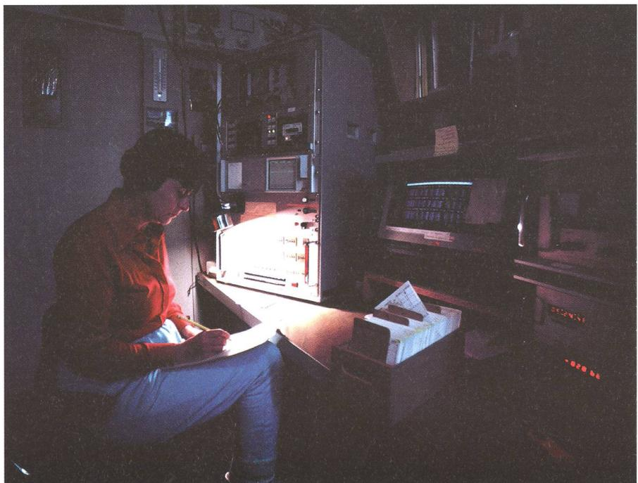
Fig. 17: Working at La Silla with P7 (photo: 1986). Data acquisition is now in digital form and telescope pointing and dome rotation are also automatic.
