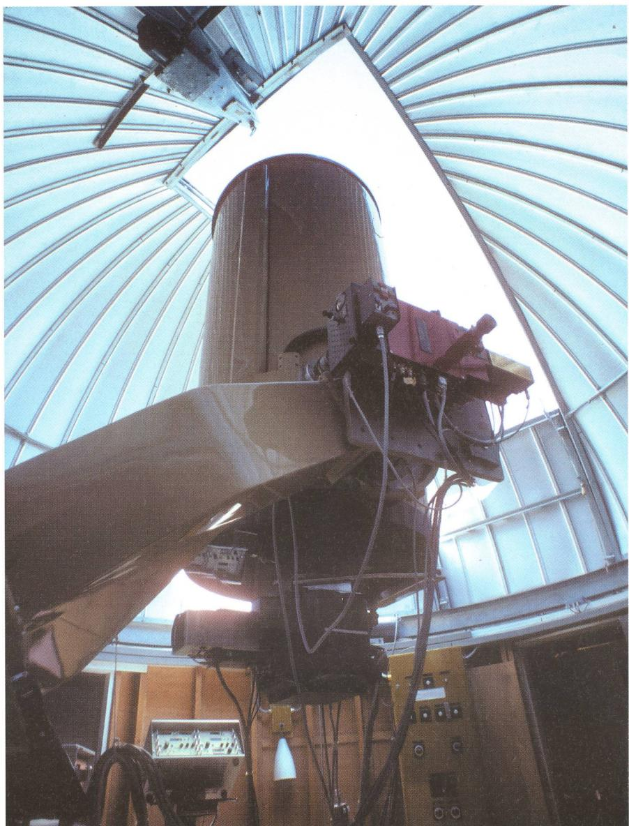
*Fig. 16: The 70 cm Swiss Telescope at La Silla equipped with the P7 photometer.*
