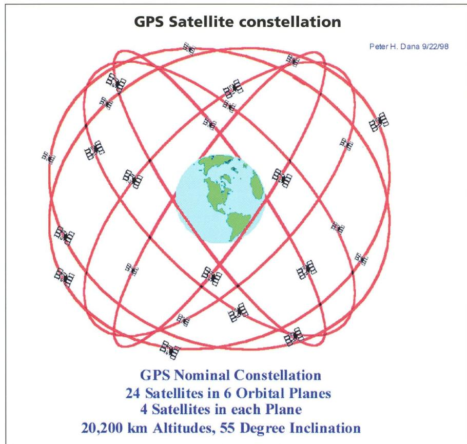
Fig. 6: Constellation of the 24 GPS satellites.
