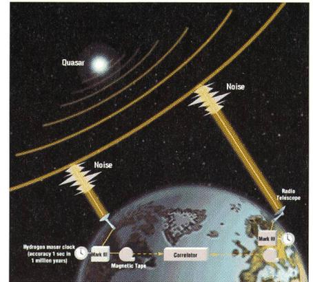
Fig. 4: Principle of VLBI.
