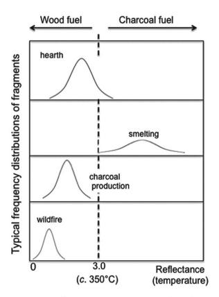
Fig. 3 – Diagrammatic fragment/temperature distributions illustrating the reflectance method.
