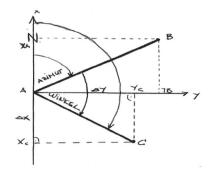
$\Delta Y = \overline{AC} \cdot \sin(Azimut + Winkel)$
