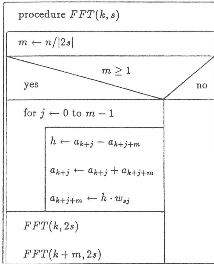
Herein  $k$  represents the index of the first element and  $n/|s|$  the order of the fast Fourier transformation.  $s$  is also needed to pick the correct unit root  $w_{sj} \stackrel{\text{def}}{=} w_n^{sj}$ . If we define  $w_l = e^{2l\pi i/n} \Big|_{-n/2 < l < n/2}$  we get
