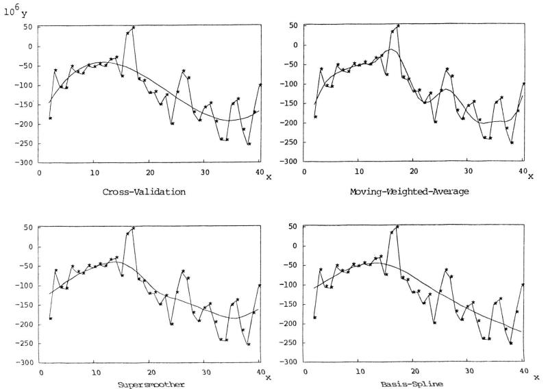
Figure 2 Supersmoother fits to the weighted residuals  $\sqrt{w_i}(y_i-\hat{y}_i)$  obtained by the four methods  $\sqrt{w_i}$   $(y_i-\hat{y}_i)$
