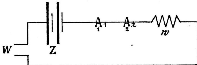
A<sub>1</sub><sup>1</sup> = Hitzdrahtampermeter
